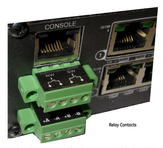
The Switch unit can receive power from either input, "A" or "B". The hub will normally draw its power from the DC source with the highest voltage at a given time.
